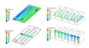
USP has unrivaled in-house CFD modeling expertise that can be used to optimize the injection, mixing and feed rates of PAA to meet the disinfection requirements of a facility.
