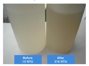
Five hours after hydrogen peroxide was added to the tower, the turbidity stabilized and the peroxide level in the bulk water was down to <20 ppm, at which point the water was evacuated from the tower to remove the solids from the system.
