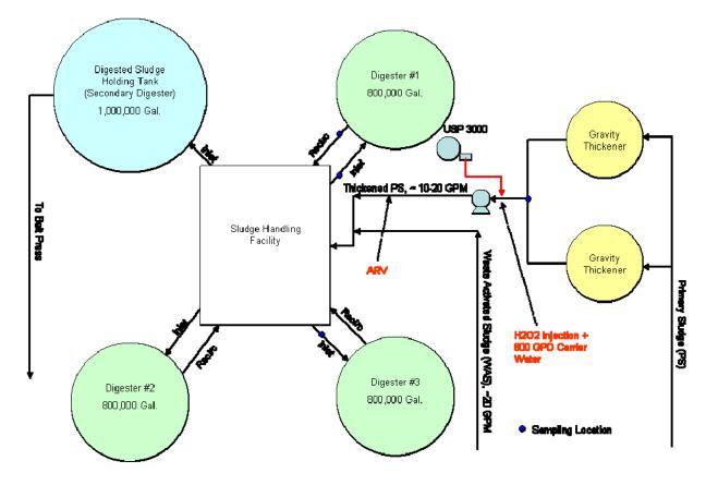
Figure 4 – Process flow diagram of the Manatee County SWWRF sludgeworks.
